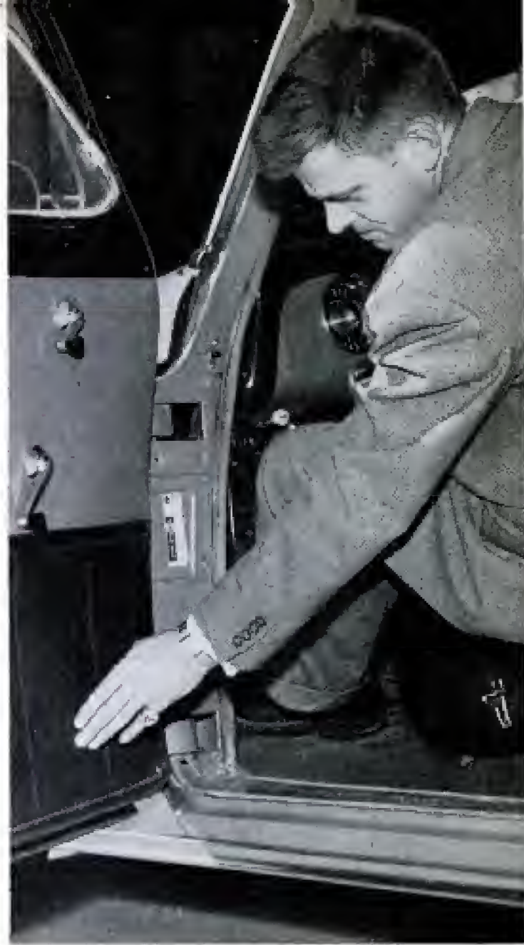
Battery and cables should be free of corrosion Brake pedal should have a maximum play of \frac{1}{4} -in.
